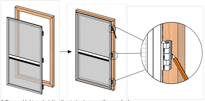
2. Disassemble hinges by taking the pivot out, remove the spare bush.
